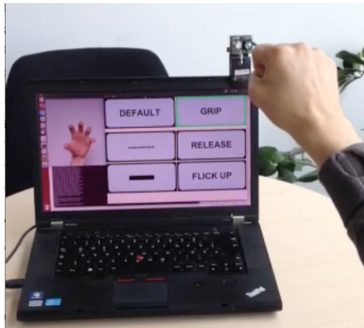
Figure 14. An exemplary hand gesture recognition setup. A user performs a dynamic gesture defined by a starting pose and an ending pose. For a dynamic grabbing gesture, pose class s_t^{start} = h (grab) starts the sequence which s_{t+m}^{end} = f (fist) ends. See Figure 6 for an overview of our ten hand pose classes. Our machine learning systems recognise the individual poses and an algorithm on top tries to identify the sequence.
