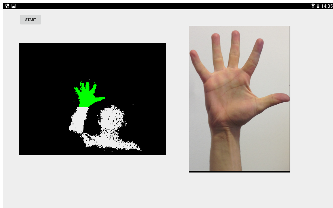
Figure 9. A demonstration of our preprocessing method. After applying a depth threshold and Principal Component Analysis (PCA), the green voxels ( left ) remain for further processing and serve to identify the correct hand posture class ( right ).
