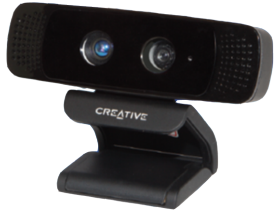
Fig. 2: The Creative Gesture Camera, capable of recording RGB images at a resolution of 640 \times 480 and depth images at a resolution of 320 \times 160 at a frame rate of 30 Hz.
