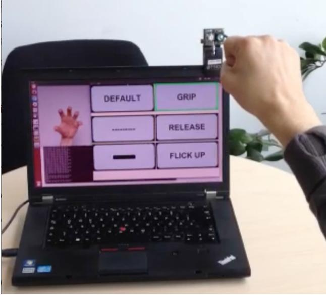
Fig. 5. Demo setup: The user performs the grabbing gesture defined by the starting pose 'h' (image), recognized by our state machine (cf. Fig.3 for notations)
