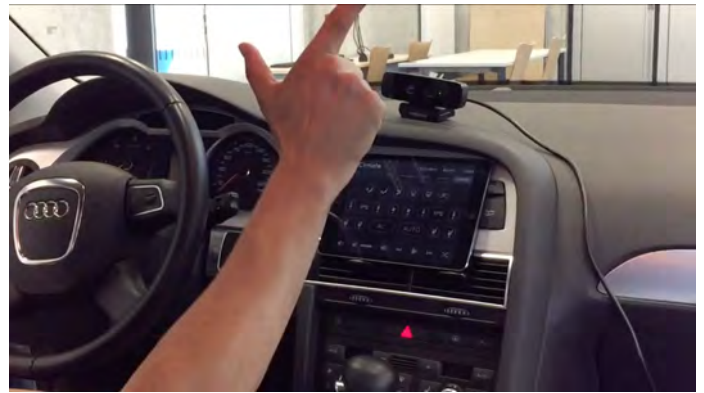
Fig. 6. Our system setup with an iPad and the Creative Gesture Camera as described in Section VI.
