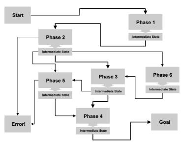
**Fig. 3.** The skill model as a network of Task Phases. The nominal path through phases 1,2,3 and 4 is emphasized using the thicker arrows.
