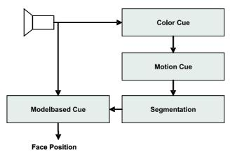
Fig. 8. Structure of the face detection module used for face finding in the camera images.
