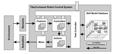
Fig. 4. The structure of a the low-level skill control system.
