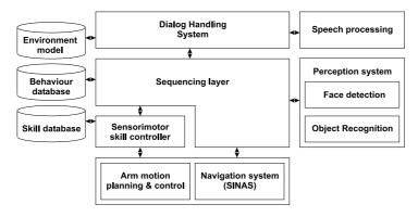
Fig. 2. The robot control system.
