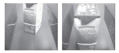
Fig. 7. The view from the gripper camera at the beginning and endpoint of the grasping motion.
