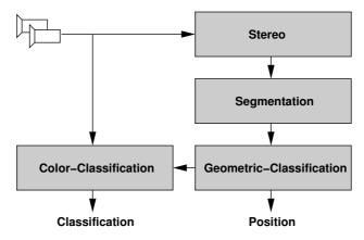
Fig. 5. The structure of the vision system used for object recognition and localization.
