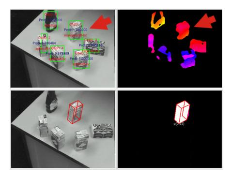
**Fig. 6.** The top left image was rectified for the stereoscopic 3D-reconstruction and the classification results are plotted into the image. The top right image shows the segmented depth data. The images in the lower row display the results of the pose and shape reconstruction.
