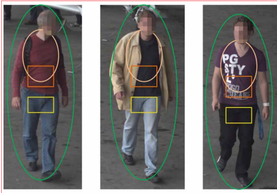
Fig. 7: The used features will be extracted from three areas which are located relative to the detection.
