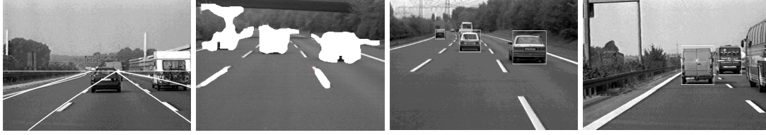
Figure 2. Lane extraction, determination of free space, and scaling estimates of vehicles using camera and environment geometry.
