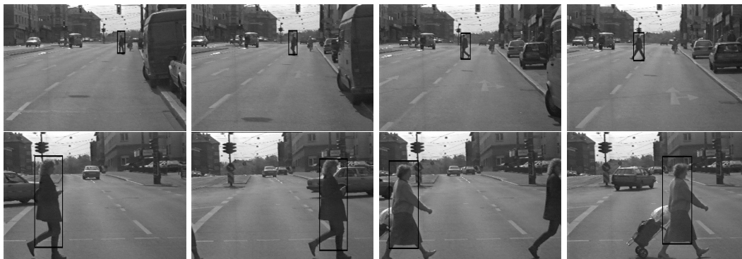
Figure 6. Tracking of pedestrians based on the cross entropy based on intensity distributions and LOC features
