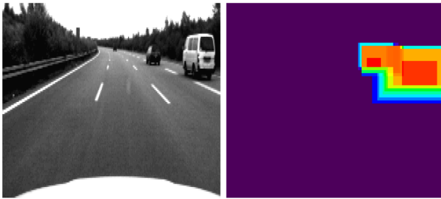
Fig. 14. Image and representation: prediction and detection of objects to be overtaken.
