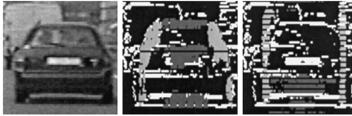
Fig. 5. Hausdorff distance classifier: each region is compared with two models.
