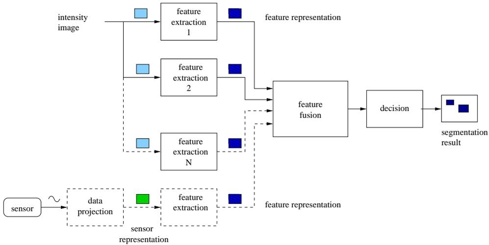
Fig. 2. Principle of a multi sensor fusion on the feature level
