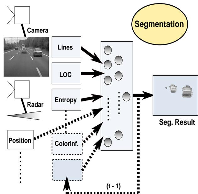
Fig. 1. Coupling model
