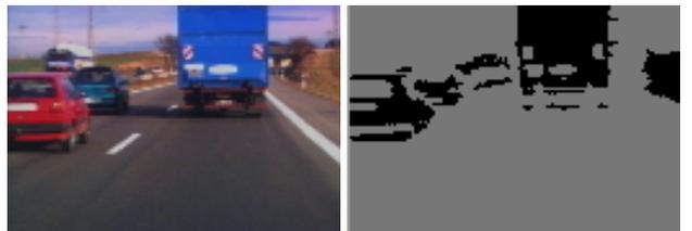
Fig. 5. original image, thresholded saturation image
