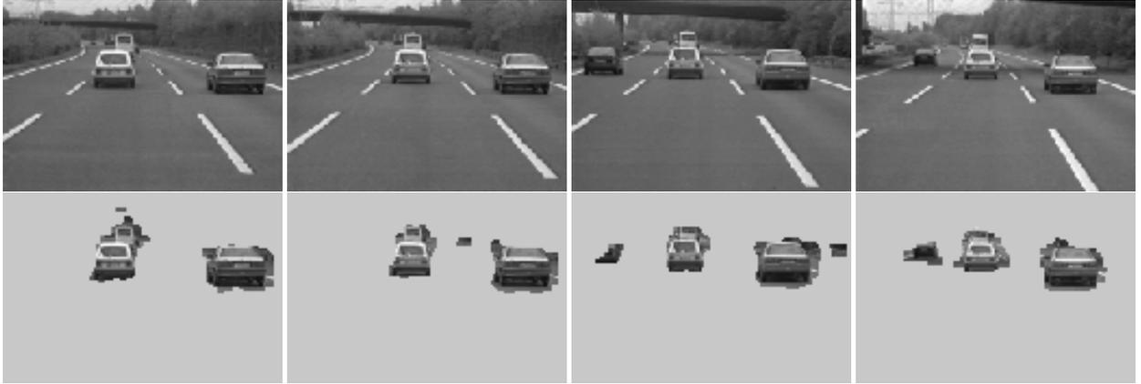
Fig. 4. Segmentation with a MLP fusion process
