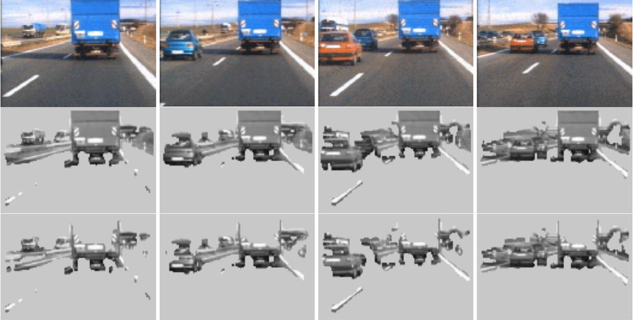
Fig. 6. Segmentation using a MLP coupling net with/without integration of saturation
