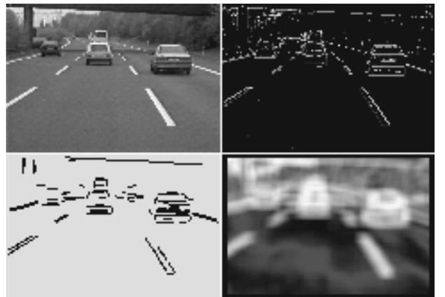
Fig. 3. Intensity, local orientation coding, polygons, local image entropy
