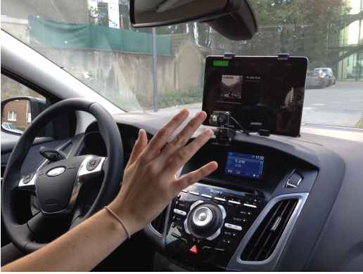
Fig. 1. Setup with ToF-sensor, Laptop and iPad in a car interior.
