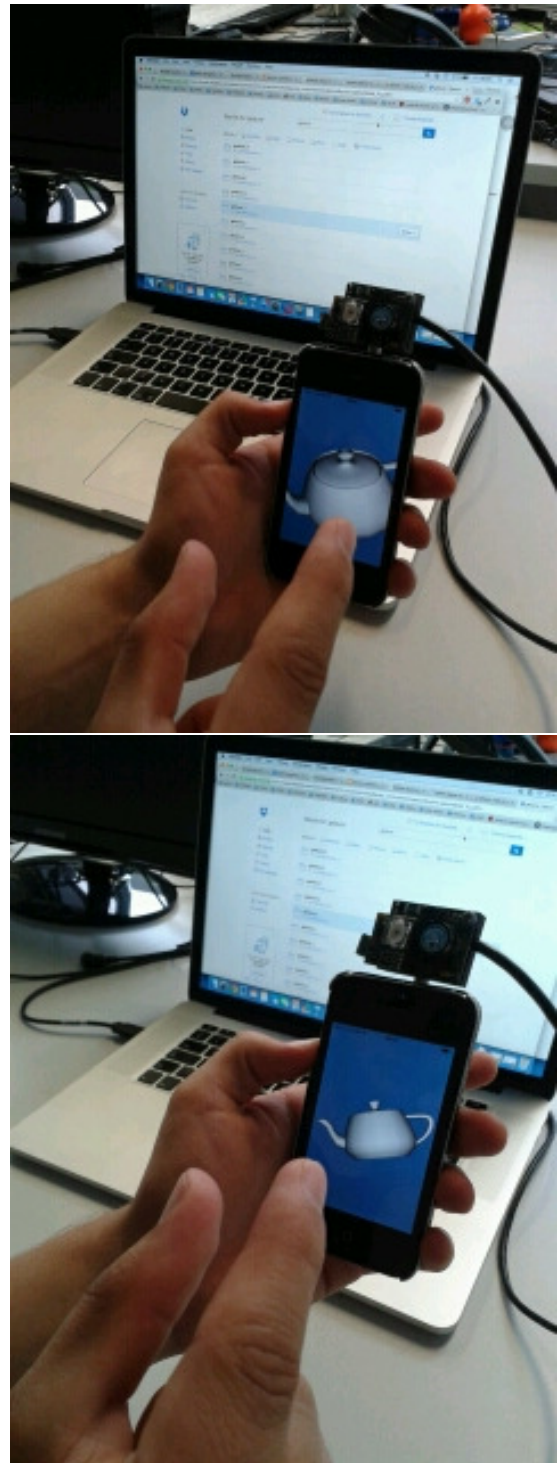
Fig. 5. Demo Application: The ToF-Sensor is mounted to the iPhone to be able to capture close-range interaction. A user zooms in on the teapot with a dynamically defined gesture.
