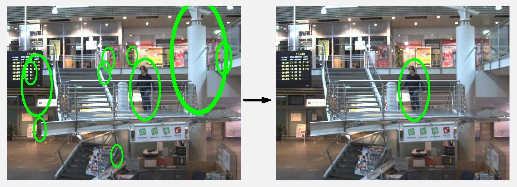
Fig. 3: Data Fusion. *Left:* Result of a person detection method with a high rate of false-positives. *Right:* Result of the fusion process. Here, the results of person detection, background segmentation and motion detection are fused which, in that case, eliminates all false-positives.
