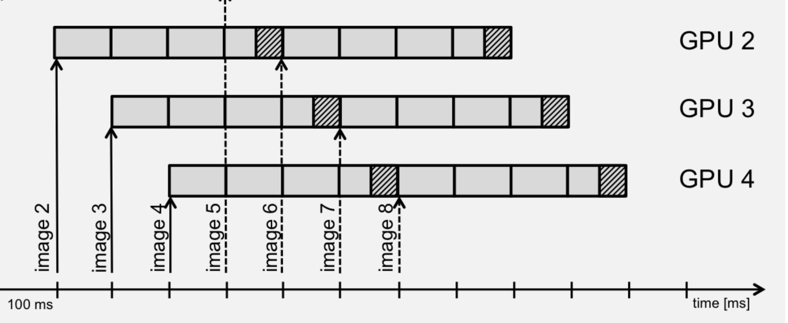
Fig. 4: Multi-Threading-Approach of a GPU-based person detection method. Each time an image is available, it is send to a free GPU which is then blocked until the processing has finished.
