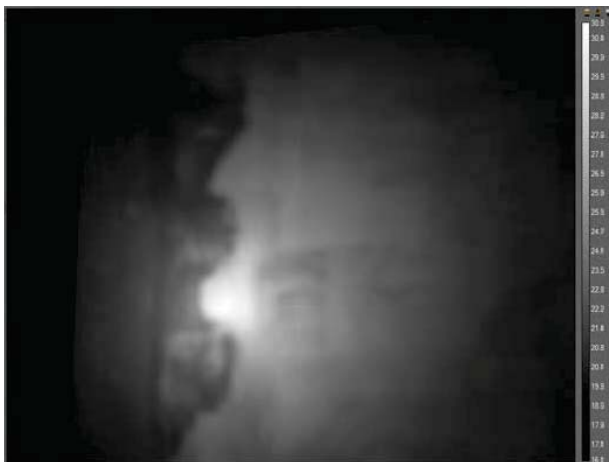
Figure 11. Glue under the surface
