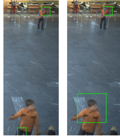
Fig. 1. Weighting of near field windows The left image shows the use of a single upper-body detector; the person in the lower part is not detected due to small amounts of candidate windows. Using transformed SVM weights, one can see on the right image that the same detector finds the person in the lower part and suppresses the small false detection now.
