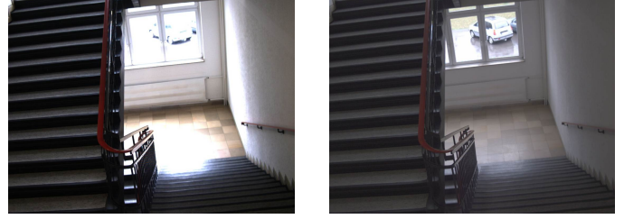
Fig. 2. Illumination correction. This figure shows an example result of the presented hardware near illumination correction. The left image is recorded without the correction and the right is recorded with the correction.
