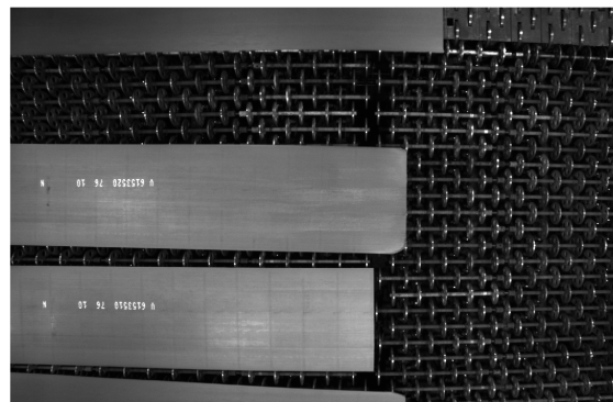
Fig. 1. Metal sheets on conveyor in cooling bed. The camera is mounted above it.
