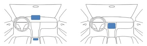
Figure 1: Typical cockpit styles: left:highly mounted display with controller, right: touchscreen
