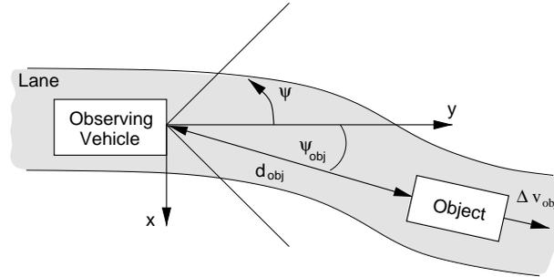
**Figure 7.** Observer-centered coordinate system for behavior planning.  $(x, y)$  determines the lateral and longitudinal position in Cartesian coordinates,  $d_{obj}$  and  $\Psi$  represent radial coordinates.  $\Delta v_{obj}$  is the relative velocity of the object.
