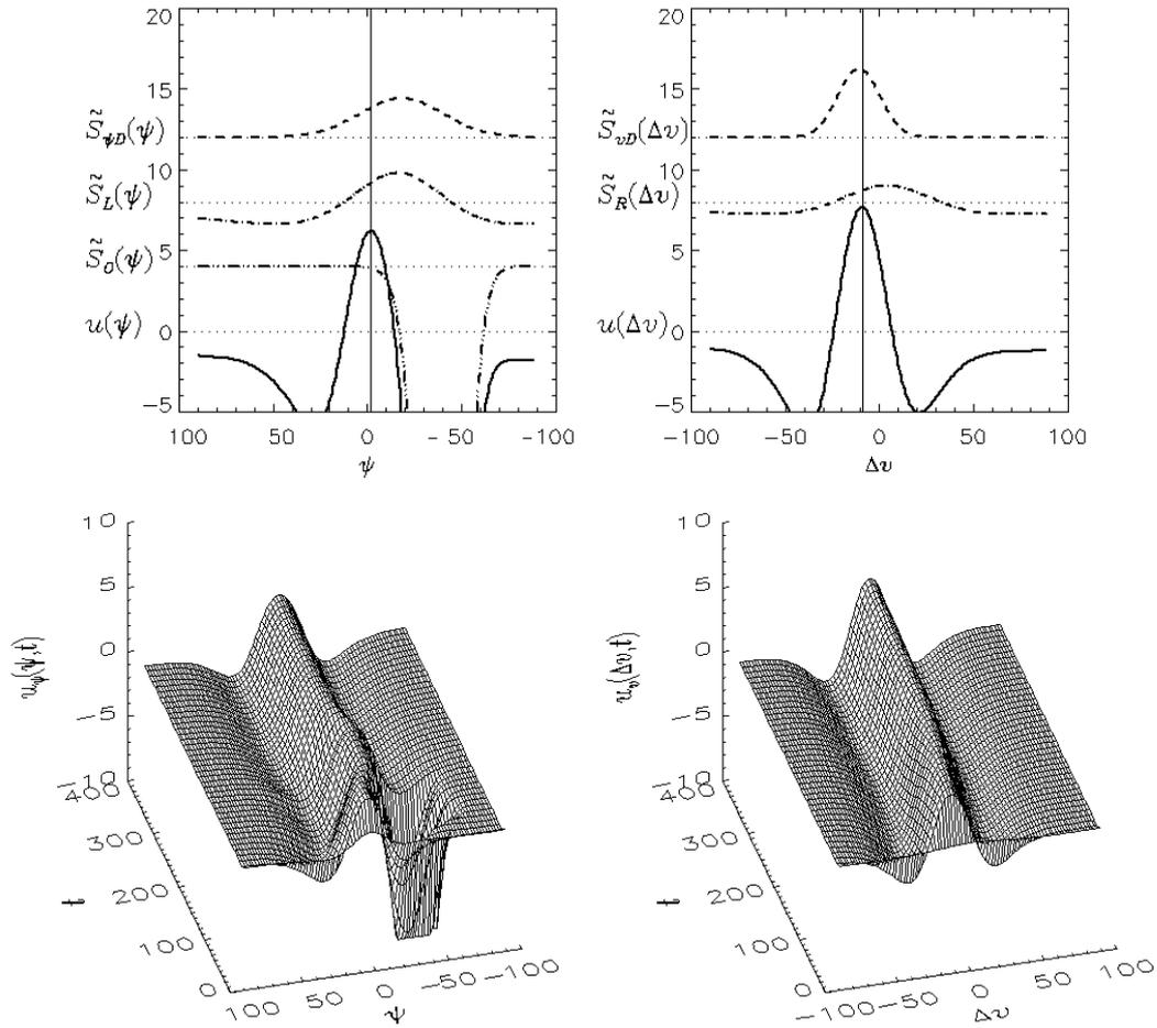
**Figure 8.** Excitation of a neural fields. Additionally the stimulus according to objects, lane, leader and intended velocity are presented (shifted to a virtual zero). Left: neural field controlling the steering angle. Right: neural field controlling the velocity.
