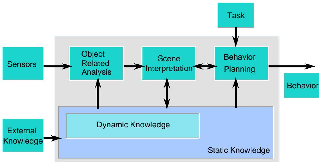
**Figure 1.** Architecture for a driver assistance system.
