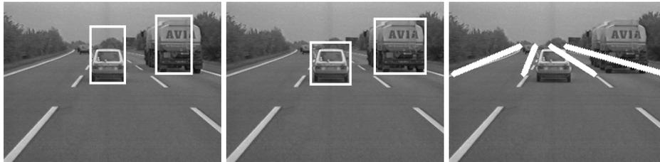
**Figure 3.** Object hypotheses generated by the object-related analysis (segmentation, tracking and lane information).
