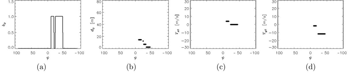
**Figure 6.** Sensor information processing. All values are determined according to angle-coordinates  $\Psi$  of the actual view. Only objects which can be observed by the sensor are included. (a) occupancy  $b_o$  of the view concerning objects (b) distance  $d_o$  to detected objects (c),(d) relative velocity of the objects in x- and y-direction
